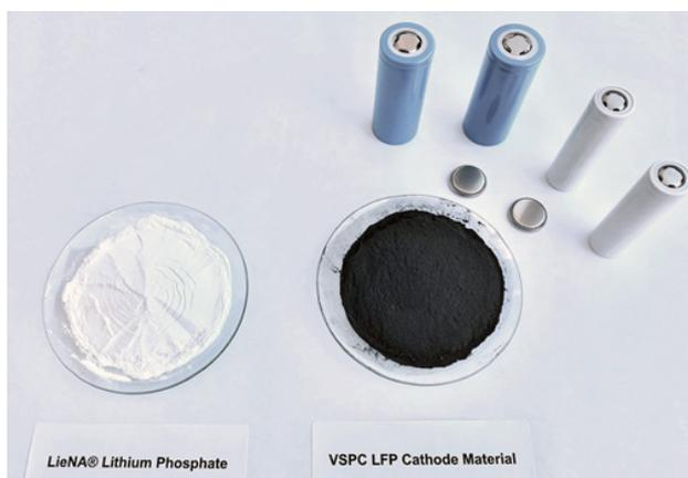
Figure 1. LFP cathode material sourced from LieNA® LP.
