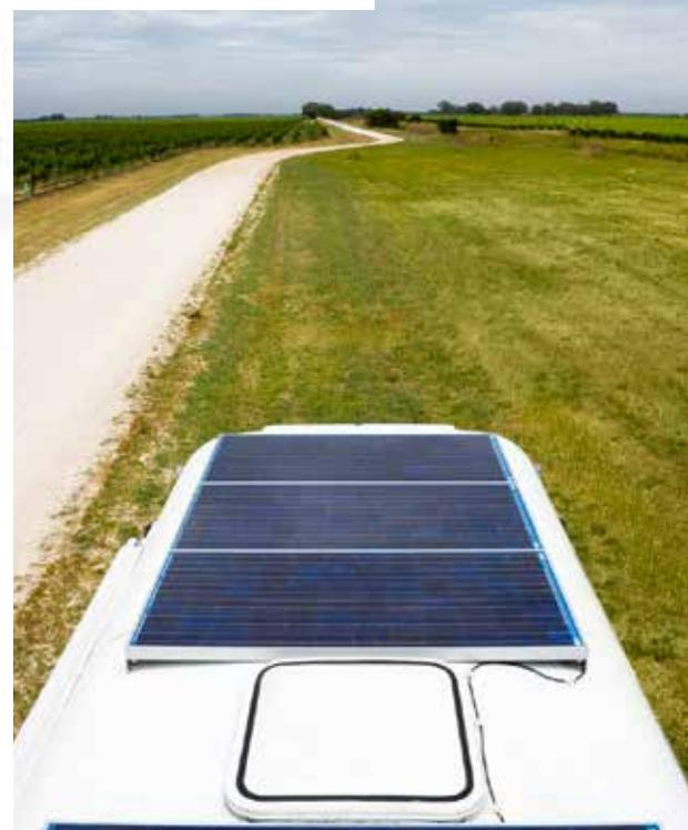
Whatever the solar option chosen, daily power needs require careful assessment first. That means checking equipment specifications, layout and any other variables likely to influence those needs. An effective power system should also allow for several days' autonomy, for back up on cloudy days or where long periods off-road prevent charging.
