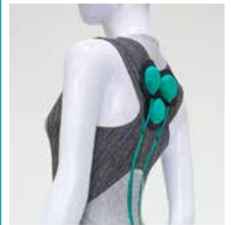
[The Aura soft exosuit for people with mobility issues. Photo courtesy of nbcnews.com .]
