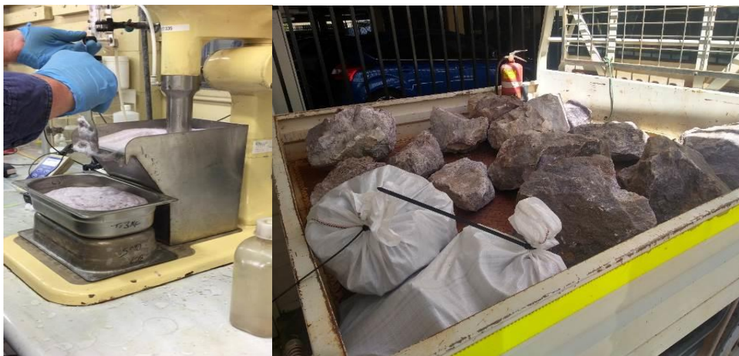
Figure 1 - Flotation test work on samples of lepidolite from a potential LSPP feed source.
