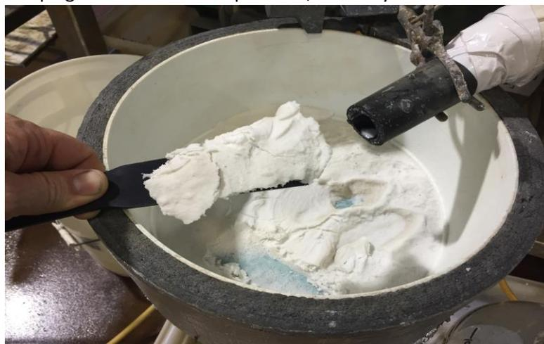
Figure 1 – Lithium Carbonate produced by the ANSTO-Minerals-run pilot plant from 10 - 13 October 2016
