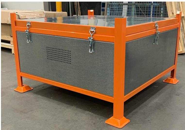
**Photo 5: Class 9 battery storage and transport stillage**
