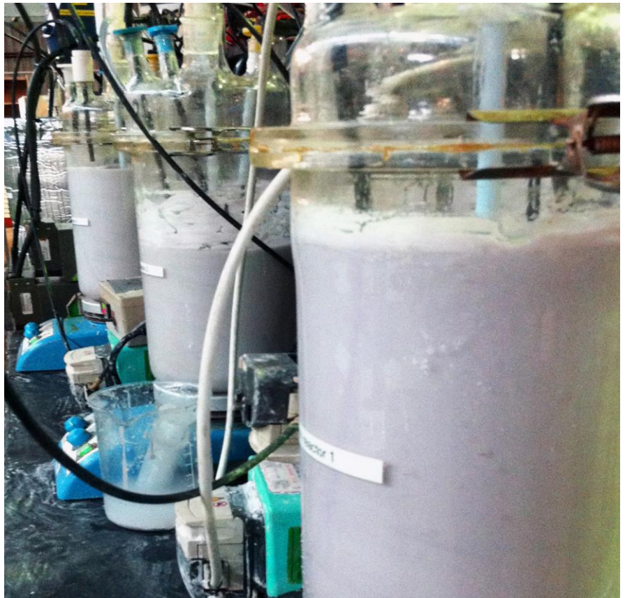
Figure 1 - Processing Lepidolite Hill lithium micas in the Strategic Metallurgy mini-plant
